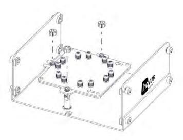
17 | Place the model mounting jig over the three columns as shown, screwing the top caps onto the columns.
