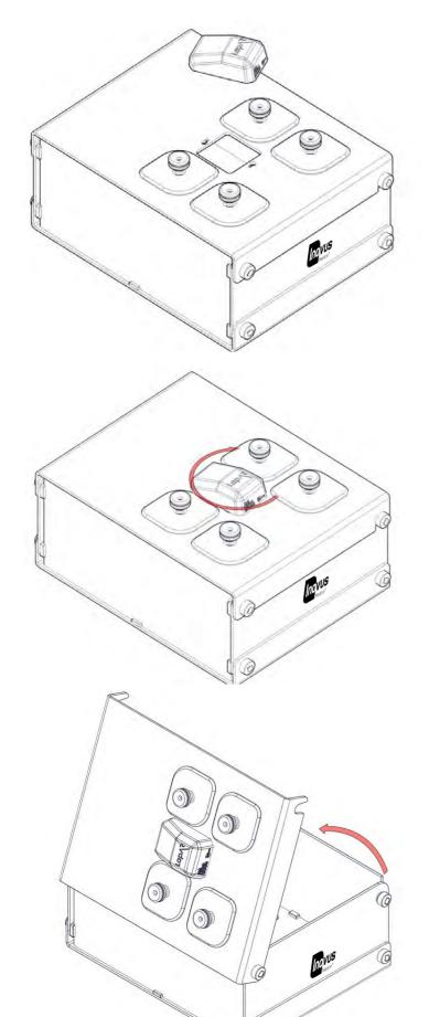
13 | Align the screws on the underside of the camera with the slots positioned on the top of the simulator.
