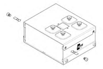
10 | Secure in place using the plastic bolts on the one side.
