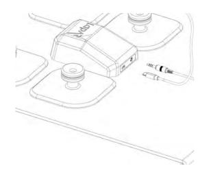
20 | Insert the camera leads (USB/USC) and model connector cable into the back of the camera.
