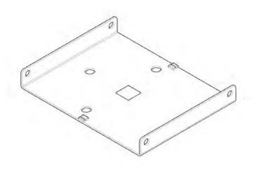
1 | When opening your simulator it is recommended that you unpack all package contents and arrange them before starting assembly. Once you have done this, take the base part as shown in the diagram and lay it on a secure flat surface.
