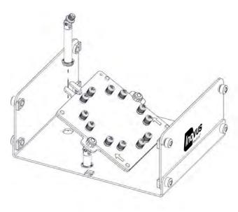
18 | To install the model mounting jig at a 45 degree angle replace the rear column with the larger one as shown.
