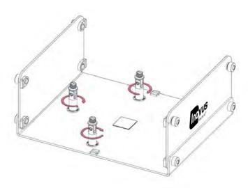
16 | To install the model mounting jig horizontally, insert the three small columns and lock in place as shown.
