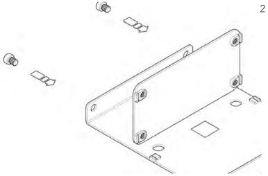
2 | Using the image as a guide, attach the rear panel ensuring the fixtures are orientated as shown.
