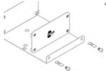
4 | Repeat the last two steps with the front panel as shown in the image. Ensure the logo is facing outwards.
