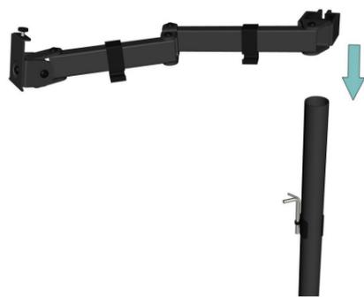
19 | The swivel arm should be pre-assembled. Slide this onto the black post.
