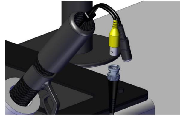
29 | Attach the BNC cable to the connector on the scope.
