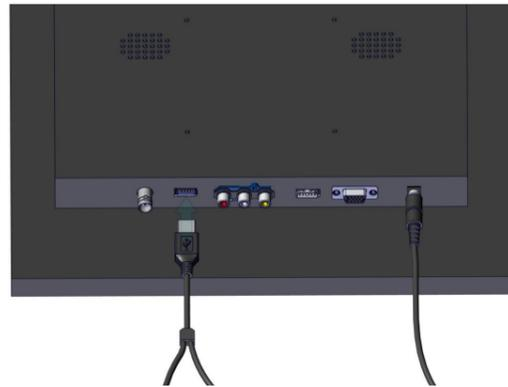
27 | Connect the USB splitter to the USB port at the back of the monitor as shown.
