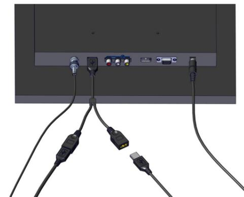
33 | Finally, connect the LED strip to the remaining USB port on the USB splitter.
