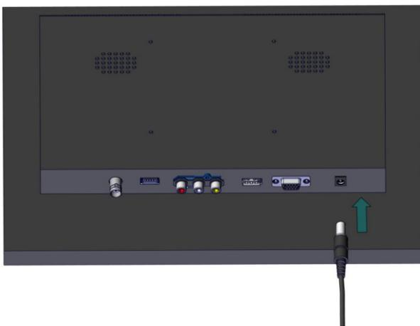
21 | All wiring can be completed using the numbered stickers attached to the ends of each adapter. For additional support, use this visual guide.
