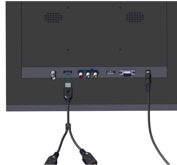
23 | Connect the USB splitter to the rear of the monitor as shown.
