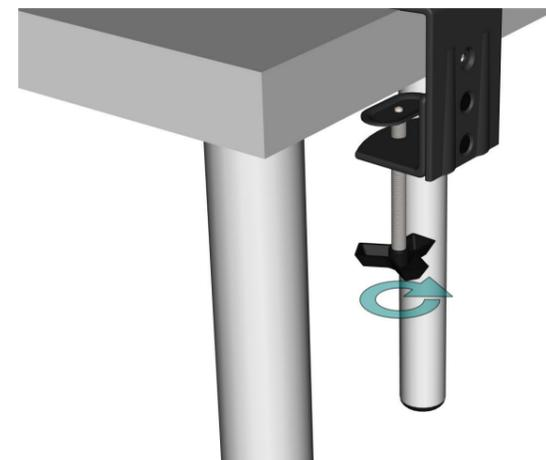
18 | With the bracket fully assembled, anchor it to your chosen work surface by turning the handle until it is tight.
