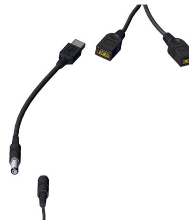
24 | Connect the USB to 5V adapter to one of the USB ports. Connect the female end of the BNC cable to the male end of the 5V adapter.
