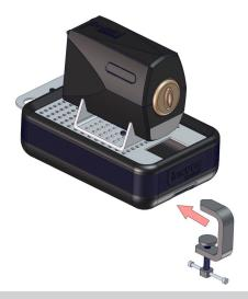
8 | Using the clamp provided, anchor the simulator at the front of the drip tray. This should prevent movement during use.
