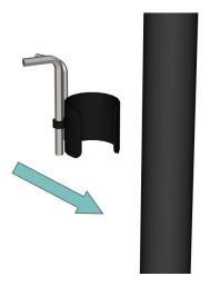
9 | Just so that we know where they are for later, identify the two Allen keys along with the push fit clamp provided. Snap this to the post and move to the next step.
