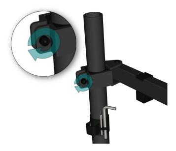
11 | At the desired height, use the largest Allen key to lock into position by turning the bolt in a clockwise direction. Once this step is complete, you may insert the end cap.
