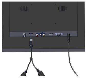
17 | Connect the USB splitter to the rear of the monitor as shown.
