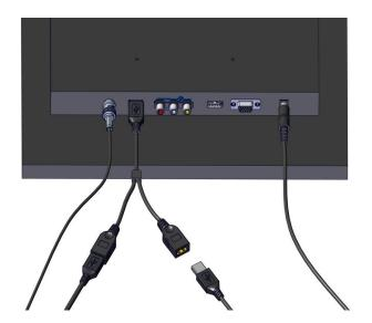
21 | Connect the USBA/B cable to the remaining USB port on the USB splitter.
