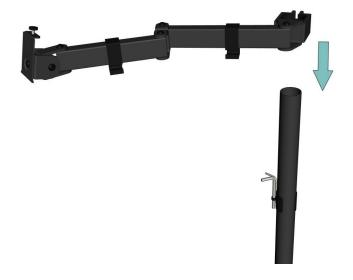
15 | The swivel arm should be pre-assembled. Slide this onto the black post, then move to the next step.
