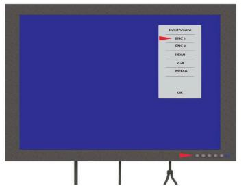
35 | In most cases, your monitor will have been pre-programmed to display the image. In the event that you do not have an image on screen, push the left most button on the screen and select BNC1.
