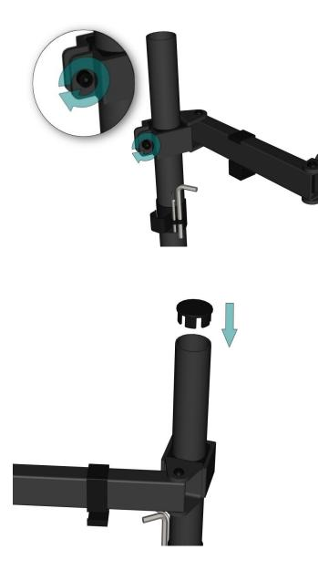
16 | At the desired height, use the largest Allen key to lock into position by turning the bolt in a clockwise direction.
