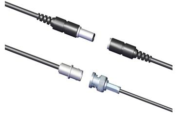
25 | Connect the female end of the BNC extender to the screen.
