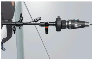
15 | Connect the endoscopic camera to the scope by pinching the two clasps.
