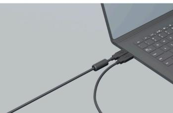
9 | Insert the light source lead into the laptop as shown.
