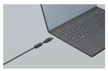
8 | Insert the USB connector into your laptop you may require use of a USBC adaptor which is provided.
