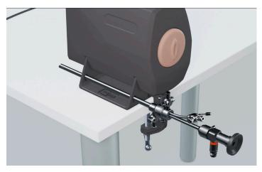
14 | You are now ready to insert the scope into the introducer. Once the scope is fully inside, ensure it is locked in place using the latch. You may use the apertures in the U-shaped bracket to hold the assembly in place as shown here.
