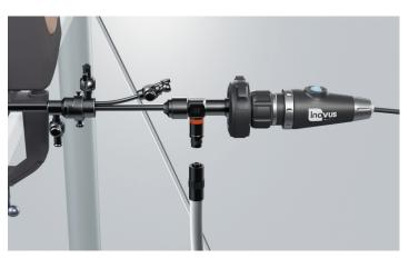
16 | Attach the other end of the fibreoptic cable to the connector on the scope by screwing it in place. At this stage, you are ready to turn the light source on.
