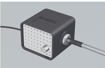
11 | Plug in the male end of the fibreoptic cable into the light source box.
