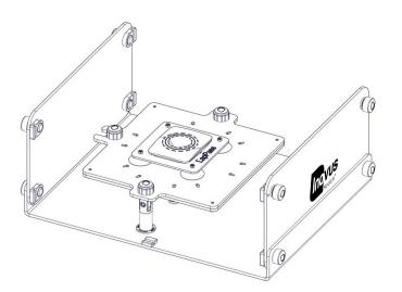
46 | The model mounting jig can also be installed upside down to act as a platform for the LapPass kit.
