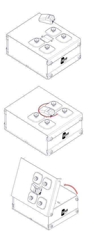
33 | Align the screws on the underside of the camera with the slots positioned on the top of the simulator.
