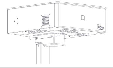
8 | Tighten all screws with allen key provided. The top box of the sim station should now be securely attached to the main column.
