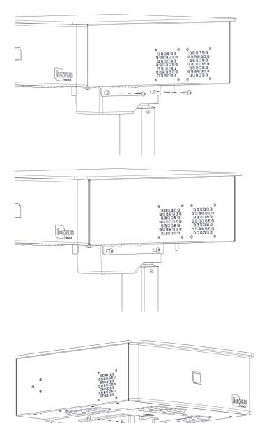
5 | Insert two bolts into the side of the LapAR Pro sim station main column and top box, screwing in place with the allen key provided.
