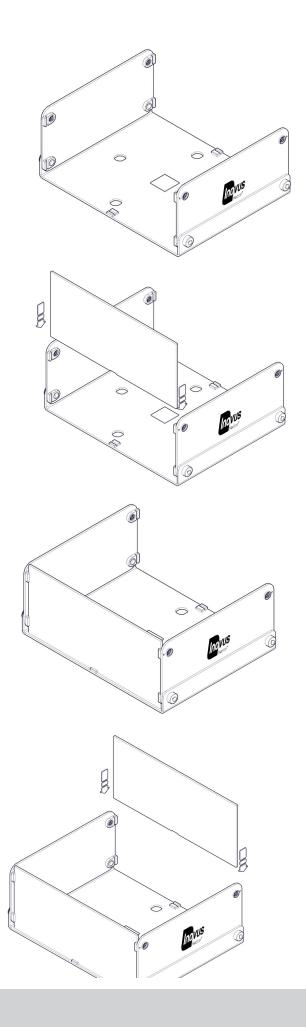
25| Once the bottom elements are secure move onto the side panels.
