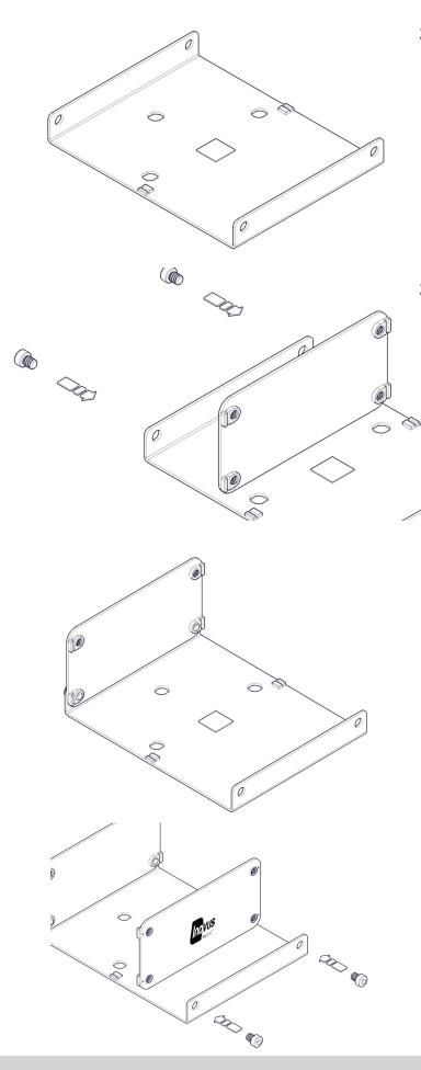
21 | Take the base part of the LapAR box trainer as shown in the diagram and lay it on a secure flat surface.
