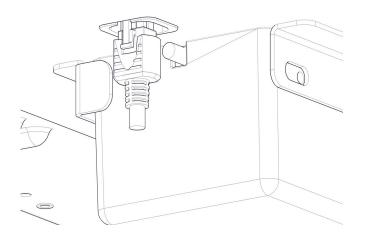
9 | Locate the main column lead on the underside of the LapAR Pro sim station box.
