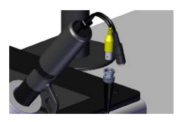
29 | Attach the BNC cable to the connector on the scope.
