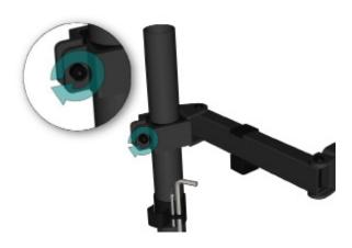
20 | At the desired height, use the largest Allen key to lock into position by turning the bolt in a clockwise direction.
