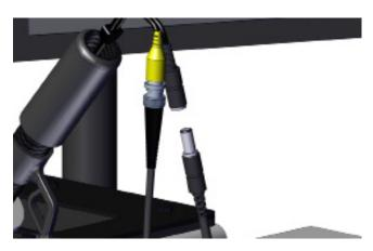
30 | Connect the remaining power cable to the female connector on the scope.
