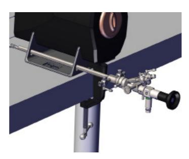
You may use the apertures in the U-shaped bracket to hold the assembly in place as shown here.
