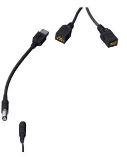
8 | Connect the USB to 5V adapter to one of the USB ports. Connect the female end of the BNC cable to the male end of the 5V adapter.
