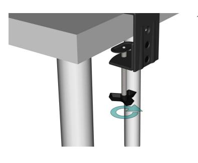
3 | With the bracket fully assembled, anchor it to your chosen work surface by turning the handle until it is tight.
