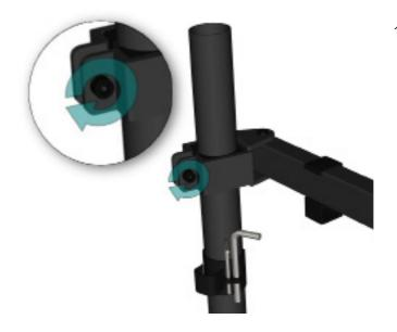
11 | At the desired height, use the largest Allen key to lock into position by turning the bolt in a clockwise direction. Once this step is complete, you may insert the end cap.
