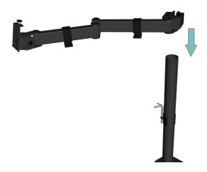
10 | The swivel arm should be preassembled. Slide this onto the black post, then move to the next step.
