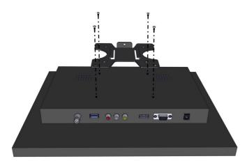
4 | Take the screen bracket and screw this to the back of the monitor using the bolts provided.
