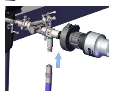
30 I Attach the other end of the fibreoptic cable to the connector on the scope by screwing it into place. At this stage, you are ready to turn the light source on.
