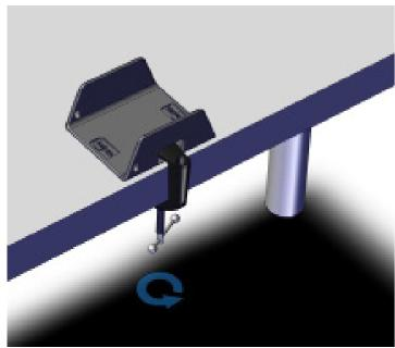
2 | Once in position, turn the handle until the clamp grips firmly to the bracket and flat surface.
