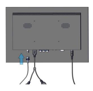
19 | Connect the female end of the BNC extender to the screen.
