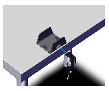
Begin by placing the U-shaped bracket on a suitable flat surface. Then, place the top portion of the small clamp through the opening at the front of the bracket, as illustrated here.
