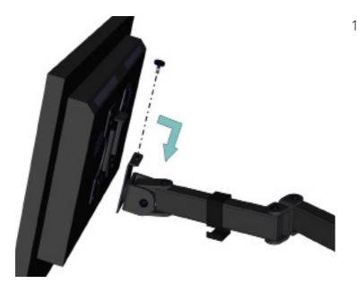
5 | Slide the monitor into position and screw the bolt into place.
