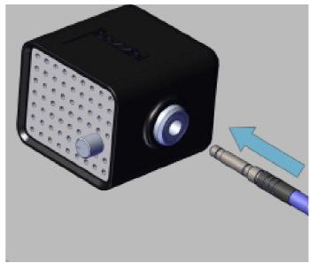
Plug in the male end of the fibreoptic cable into the light source.
