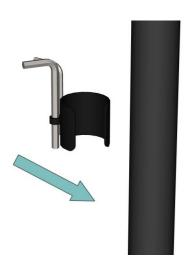
9 | Just so that we know where they are for later, identify the two Allen keys along with the push fit clamp provided. Snap this to the post and move to the next step.
