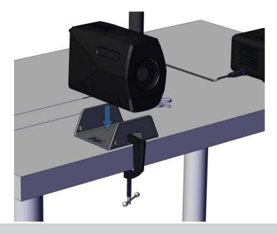
3 | Place the retaining case onto the U-shaped bracket as shown.
