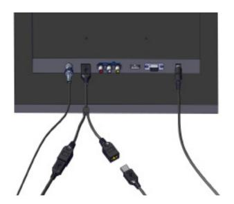
Connect the USBA/B cable to the remaining USB port on the USB splitter.
