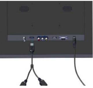
7 | Connect the USB splitter to the rear of the monitor as shown.
