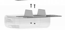
4 | Use the remaining bolt and nut to secure the acrylic plate at the rear of the drip tray. This ensures that the plate remains stationary whilst the simulator is in use.
