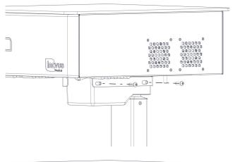
5 | Insert two bolts into the side of the sim station main column and top box, screwing in place with the allen key provided.
