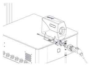
24 | Attach the fibre optic light lead to the scope.
