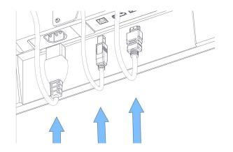
27 | Plug the 3 cables into the relevant ports in the underside of the monitor.
