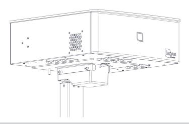
8 | Tighten all screws with allen key provided. The top box should now be securely attached to the main column.
