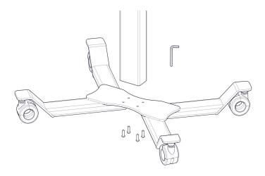
2 | Start the assembly of your sim station by screwing the 4x bolts into the underside of the base. You can do this using the allen key provided.
