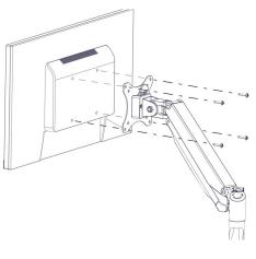
17 | Locate 4x bolts and thread through the bracket and into the back of the monitor.
