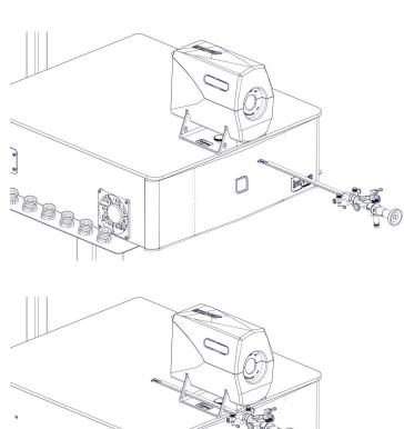
21 | Insert the scope into the introducer.
