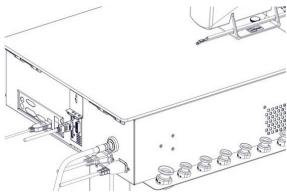
26 | Plug the power cables into the relevant ports at the back of the sim station as shown. (Please note the monitor stand is not shown here just for clarity of plug positioning).
