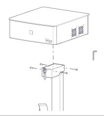
4 | Locate the 4x bolts provided to attach the top box.
