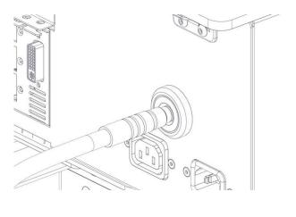
25 | Insert the fibre optic light lead into the back of the sim station.
