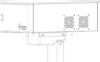
6 Ensure the bolts are finger tightened initially whilst you move onto the next step.
