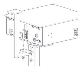
11 | Taking the Z-shaped monitor bracket, attach to the underside of the top box of the sim station using the 2x nuts provided.
