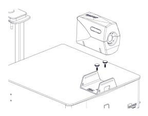
19 | Align the U-shaped bracket with the bolt holes on the top of the sim station and secure using the thumb screws provided.
