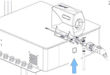
28 | Turn the system on using the power switch on the front of the sim station. Once the computer has loaded up, select the HystAR icon on the touch screen monitor and follow the instructions inside the software.
