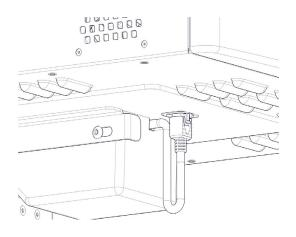
10 | Secure the lead in place with the connector as shown.
