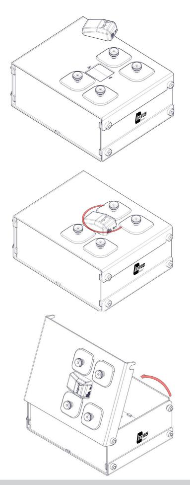
13 | Align the screws on the underside of the camera with the slots positioned on the top of the simulator.
