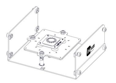
25| The model mounting jig can also be installed upside down to act as a platform for the LapPass kit.
