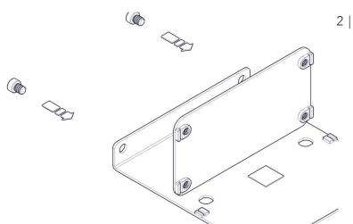
2 | Using the image as a guide, attach the rear panel ensuring the fixtures are orientated as shown.
