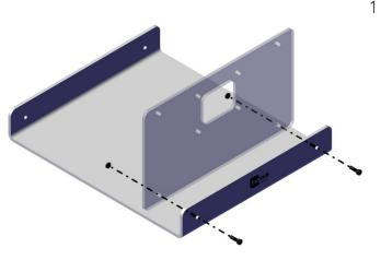
1 | Begin the assembly by taking out parts 00000917 and 00000328. Using 2 x 00000640 bolts and 2 x 00001159 nuts, screw the 00000328 panel into position as shown.
