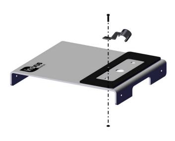
7 | Use the remaining 00000640 bolts and 1 x 00001159 nuts to position the camera bracket (00000338).
