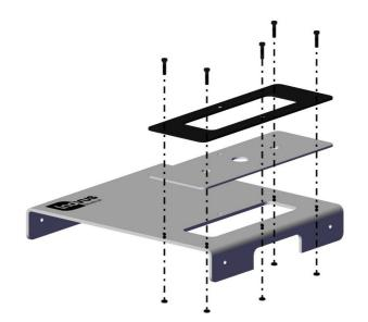
5| You may now start the top panel subassembly. Taking 00001201, 00000170 and 00000171, secure as shown using 5 x 00000640 bolts and 5 x 00001159 nuts.
