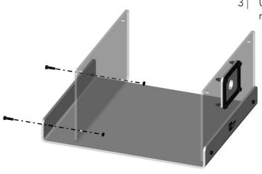
3 | Using 2 x 00000640 bolts and 2 x 00001159 nuts, secure the rear panel 00001457.
