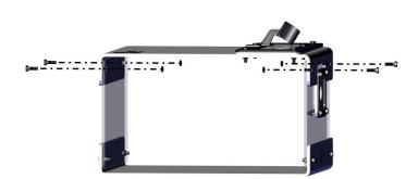
9 | Using 2 x 00000640 bolts & 2 x 00001159 nuts, secure it to the upright panels.
