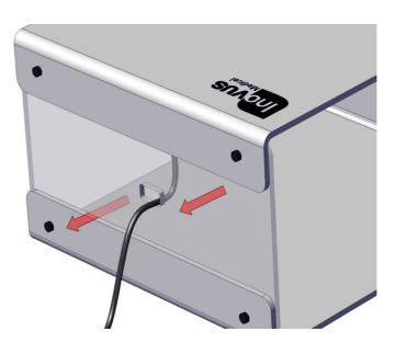
11| Feed the USB cable through the aperture in the rear panel as shown.
