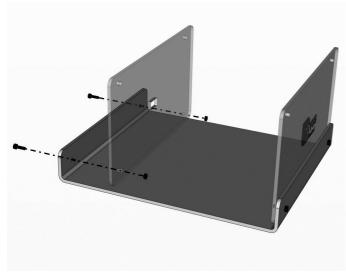
2 | Using 2 x 00000640 bolts and 2 x 00001159 nuts, secure the rear panel 00001458.
