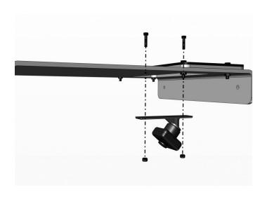
7 | Use the remaining 00000640 bolts and 2 x 00001159 nuts to secure the camera unit to the underside of TPB01.
