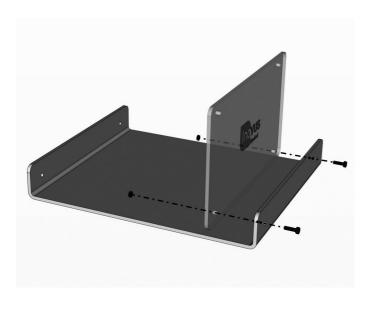
1 | Begin the assembly by taking out parts 00001213 and 00001212. Using 2 x 00000640 bolts and 2 x 00001159 nuts, screw the 00001212 panel into position as shown.
