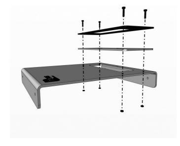
4 | You may now start the top sub-assembly. Taking parts numbered 00001204, 00000170 and using 00001204 and 00000171, secure as shown by using 4 x 00000640 bolts and 4 x 00001159 nuts.
