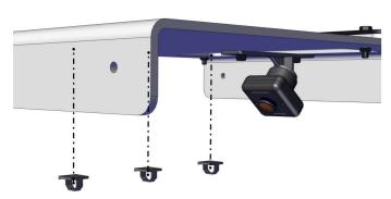
8 | Position the adhesive wire clips in line with the camera unit on the underside of TPB01.
