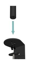
17 | Using the three black bolts provided, attach the black post to the C-clamp.
