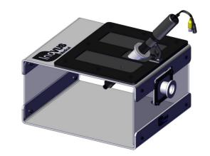
4 | Should you place the scope into the top port, you may anchor it in position by placing it into the cradle of the scope bracket. This is particularly useful for solo training.
