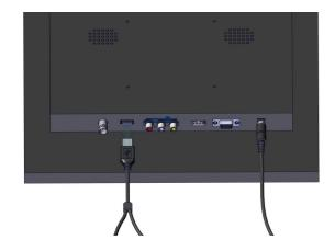
27 | Connect the USB splitter to the USB port at the back of the monitor as shown.
